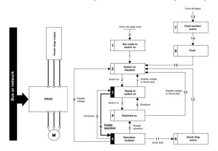
**NOTE:** It is possible, but not necessary to apply the 3 - Switch on command followed by the 4 - Enable Operation command to switch successively into the operating states 3 - Ready to Switch on, 4 - Switched on and then 5 - Operation Enabled. The 4 - Enable operation command is sufficient.
