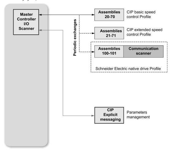
The DeviceNet fieldbus module is compliant with the ODVA drive profile. It supports the following profiles:
