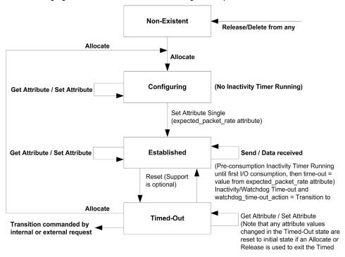
**NOTE:** The allocate and release services send the connection instance back to initial state. All object attributes are reset to their default values.
