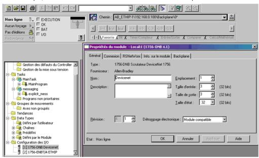
The DeviceNet module is identified with the symbol: **Module\_DNET** . This identifier will be used later with tools like the class instance editor.
